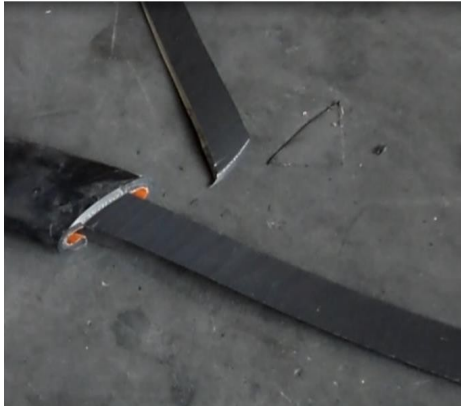
Extraction of iron core after cutting the damaged part
