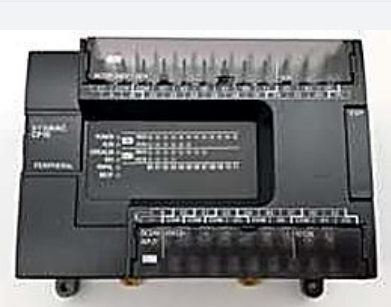
티센벨리노 호환 PLC SYSMAC CP1E-E30SDR-A
